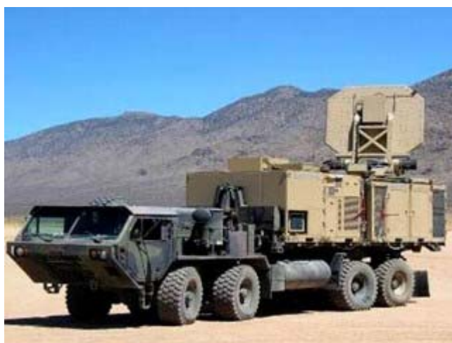
An operational version of the Active Denial System is shown. It is an invisible, counter personnel, directed-energy weapon. (U.S. Air Force )
